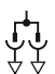
Cable connection with outside-cone plug (not included in the scope of supply)
